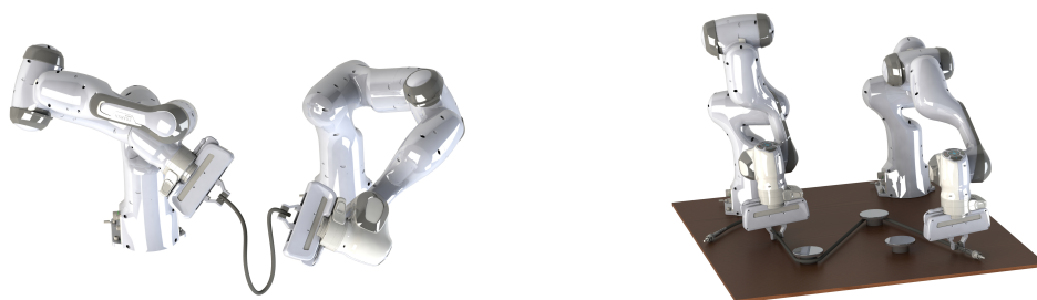
Figure 1: Studied scenarios of dual-arm manipulation of deformable objects.
