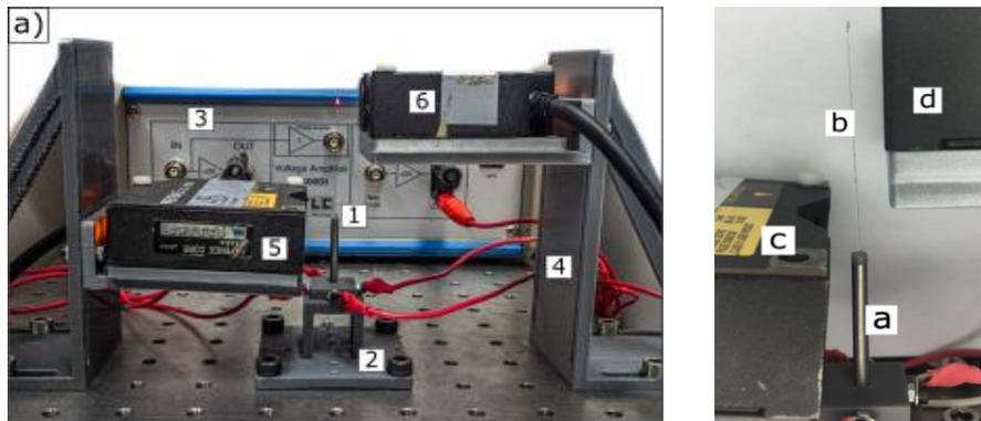
Left figure: 1. Piezoelectric tube actuated optical fiber; 2. Support base; 3. Voltage amplifier; 4. Sensors bases; 5&6. Displacement sensors. Right figure: a. Piezoelectric tube actuator; b. Optical fiber; c&d. Displacement sensors (the same as 5&6 in left figure)
