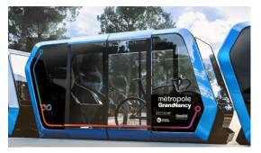
While the work has just begun for the implementation of a first 2.2 km loop allowing the circulation of 10 pods for the Paris 2024 Olympic Games, Urbanloop is facing new challenges for a city-wide installation. This scaling requires improving the performance of individual pod control and addressing issues related to a large number of pods on the circulation loops. The
