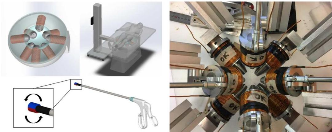
Figure 1. (a) Conceptual illustration of the electromagnetic system and laparoscopic magnetic tool for the magnetic navigation and control of magnetic microrobots for drug delivery.(b) Experimental medical electromagnetic platform that has been developed.
